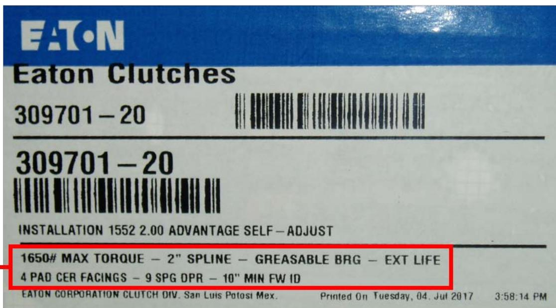
This misprinting does not affect product performance. Box labels are printed with correct part numbers and clutches are properly manufactured, but labels may be printed with an inaccurate description of the clutch within. Use the [Eaton Clutch Selector \(CLSL1511\)](#) for correct product descriptions.
